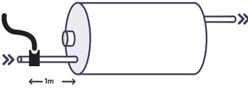
Plumb valve inline to inlet pipe at least one meter from geyser.
