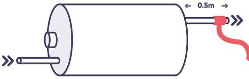
Strap cable to hot water outlet pipe 0.5m from geyser.
