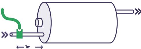
1. Plumb flow meter to inlet pipe at least one meter from geyser.
