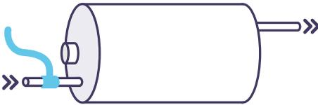
Strap to cold water inlet pipe as close as possible to the geyser.
